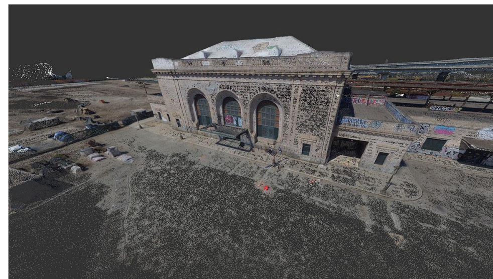
A point cloud is displayed in Autodesk ReCap
